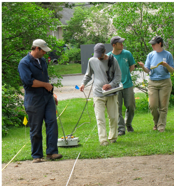
Figure 1.11. Drs. John Steinberg and Brian Damiata performing a GPR survey at Gore Place using a Måla X3M system..
